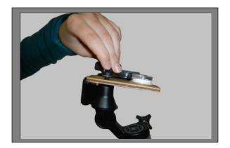
Attach the digital camera to the Bogen-Manfrotto 3025 3D junior tripod head.
