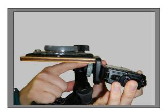
Attach the digital camera to the Bogen-Manfrotto 3025 3D junior tripod head.
