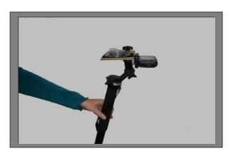
The camera has to be vertical, pointed towards the ground (a bubble level will indicate whether it is at the right angle or not)
